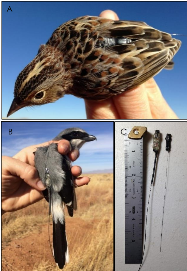
Figure 16: A) A grasshopper sparrow and B) loggerhead shrike outfitted with radio-transmitters. C) comparison of shrike (left) and sparrow/pipit (right) transmitters. Photos by Erin Strasser.
