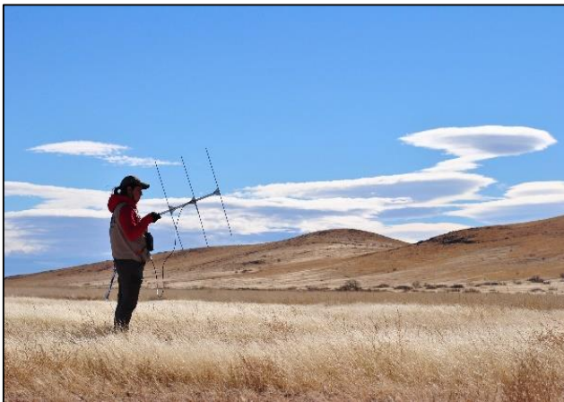
Figure 18: Handheld and truck-mounted antennas were used to track radio-tagged birds. Photos by Denis Perez and Erin Strasser
